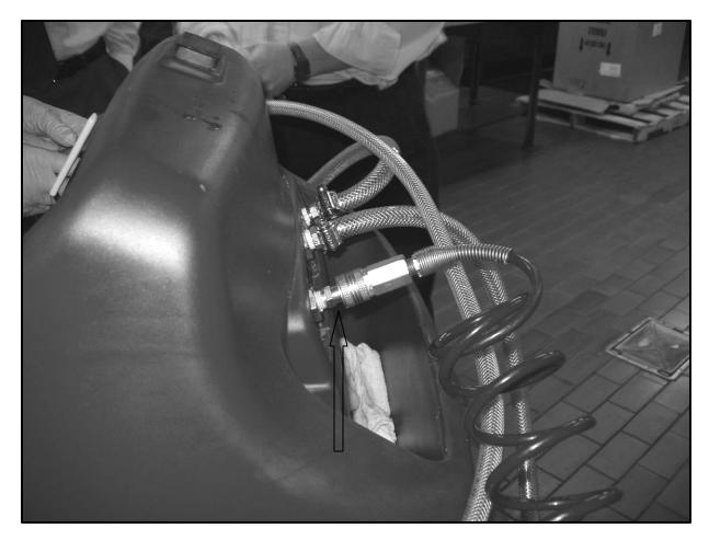
Connect unit to shop air supply - (no min. max. spec at present)
